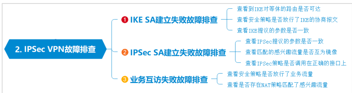
图14-17 IPsec VPN 故障排查思路
