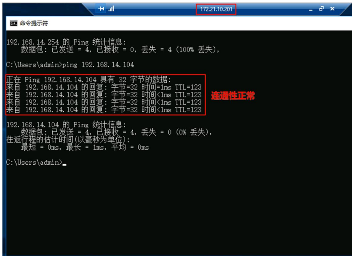
图6-24 IPSec VPN 业务连通性测试
